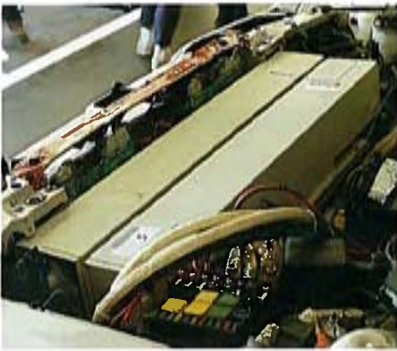
With the engine removed, the two 5 watt argon lasers fill the top half of the under bonnet space.
